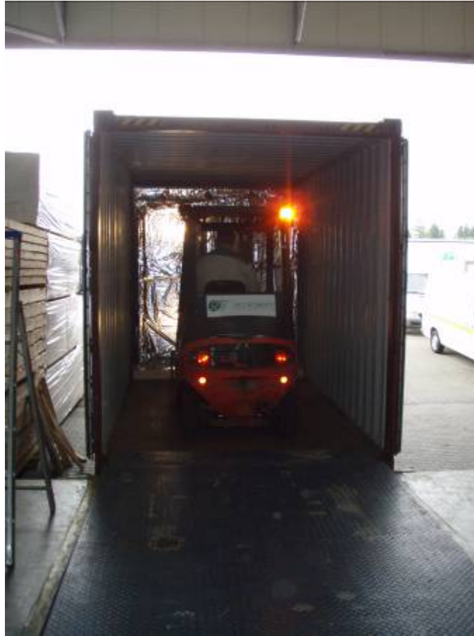
Figure 6.3.9.1b: Module removal from sealed Iso container using forklift.
