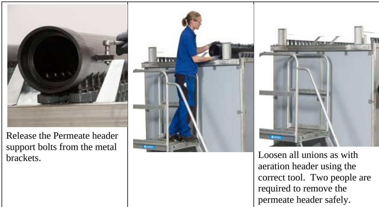
Figure 10.1.3a: Header Disassembly
