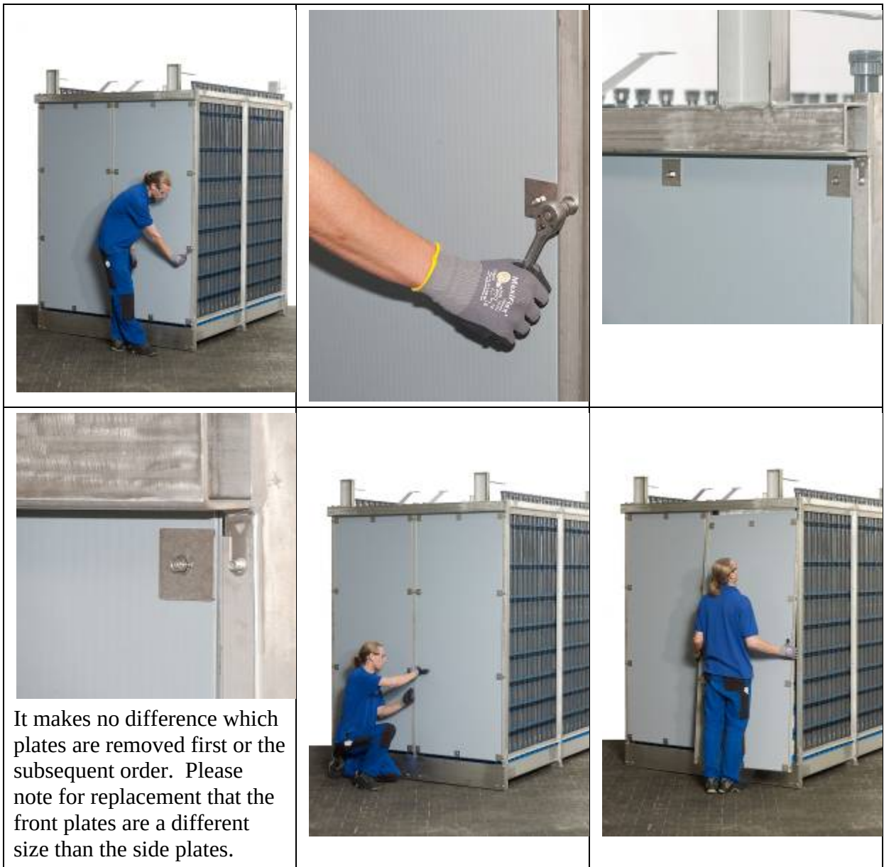
Figure 10.1.3c: Module Plate Removal
