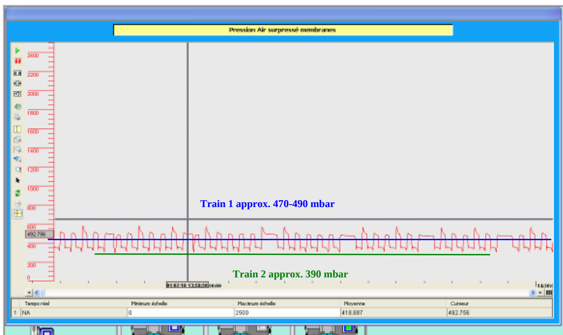
Figure 7.2.2.2 Blocked Aerator Automatic Recovery with Power Flush Improving
